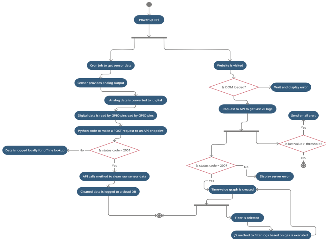
Fig. 1 High-level design of air quality monitor
